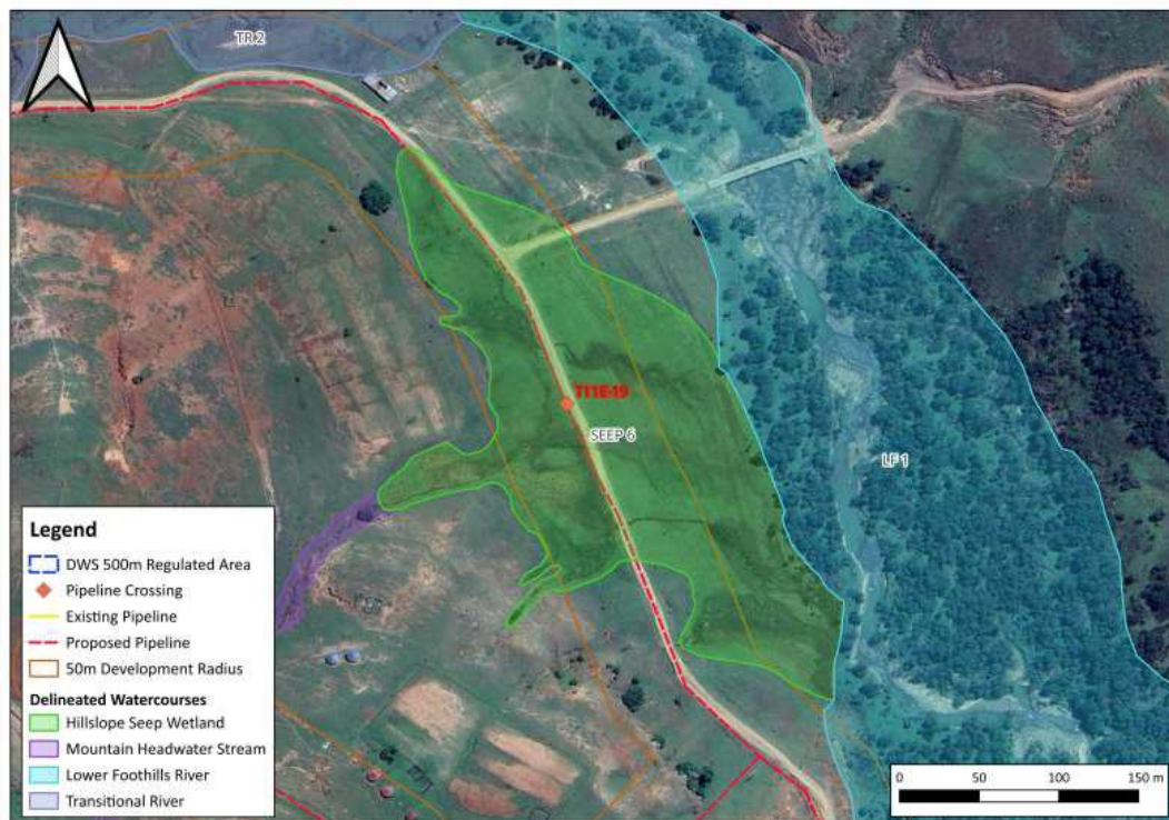
Figure 20: The proposed pipeline alignments in relation to the delineated aquatic ecosystems, specifically SEEP 6 (Ellery, 2025).
